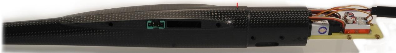
Bring the receiver antennas to the outside of the red mark.
